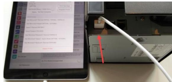
First select the **Star Micronics Lightning (USB) Thermal (TSP143IIIU)** option. Using a standard iPad lightning cable, you can plug your iPad directly into the TSP143IIIU's 5V USB port.
