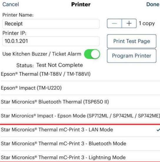
To support each mC-Print3 interface, we've added mC-Print3 mode options on the **Printer** setup screen.
